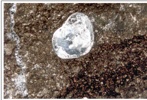
TS WA-17/7b 13x XN N35720 Micrite is dolomitised leaving bioclasts intact.
