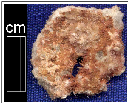
Rosette of barite, clay and gypsum (inner sample WA17/15).
