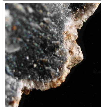
Edge view, sample WA17/14 showing how the crystal coating only coats the surface and does not penetrate deeply into the bedrock.
