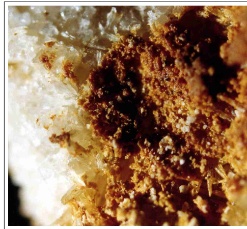
Needle crystals resemble aragonite but no aragonite was detected. Sample WA17/15, x25.
