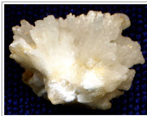
Osborne sample B69 (cut, 5 mm wide) has aragonite and huntite interior and calcite coating.
