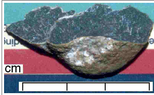
Specimen WA17/14 looks corroded from the outside but inside the limestone is intact. Vein contains barite.
