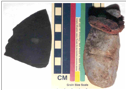
Cut specimen: WA17/7 black limestone, grey on weathered surfaces. Chert is rusty.
