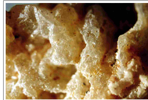
Sample WA12/15 at S5: Underside of coating forms overlapping scales. Width of view is about 5 mm
