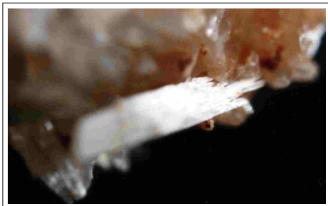
Sample WA12/17: Tattered crystal terminations. Width of view about 0.5 mm.
