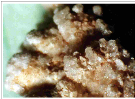
Sample WA12/14. Underside of part of “tray” speleothem at S5. Width of view is about 4 mm.
