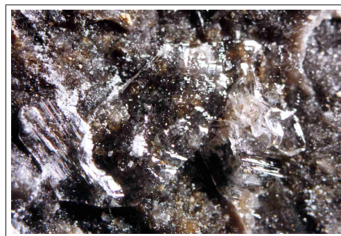
Surface of sample WA17/2, site S2, shows barite and gypsum crystals.
